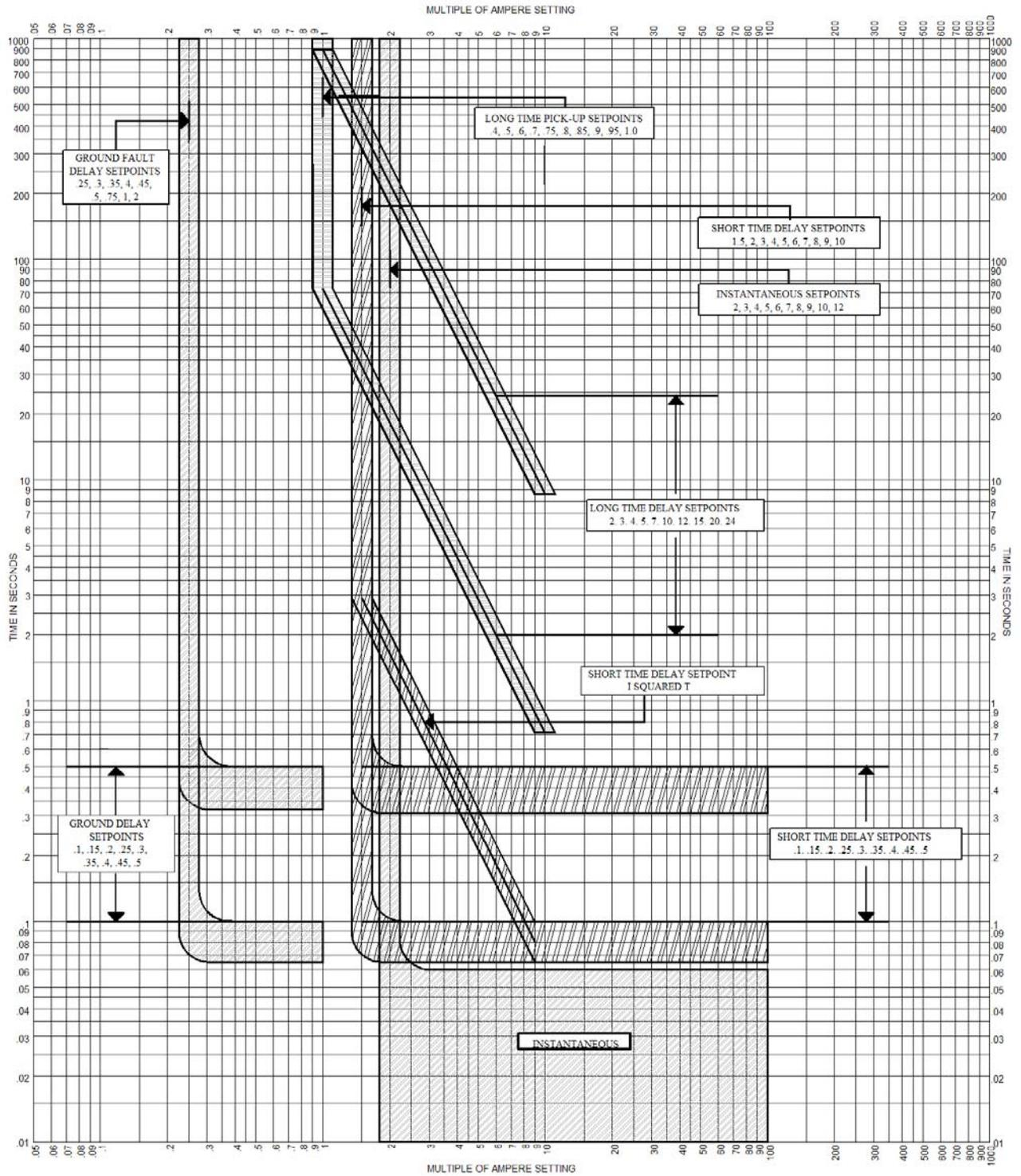
RMS-2007AF PROGRAMMABLE LOGIC CONTROL Rev.01 TIME-CURRENT CHARACTERISTIC CURVES
