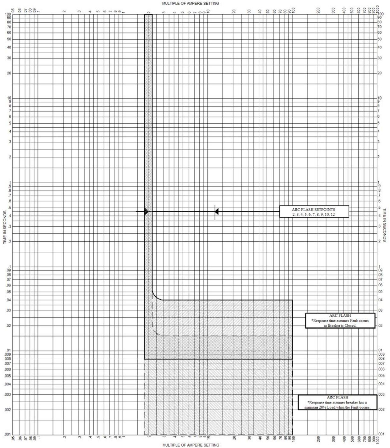
SURE-TRIP RMS-2007AF PROGRAMMABLE LOGIC CONTROL Rev.01 TIME-CURRENT CHARACTERISTIC CURVES
