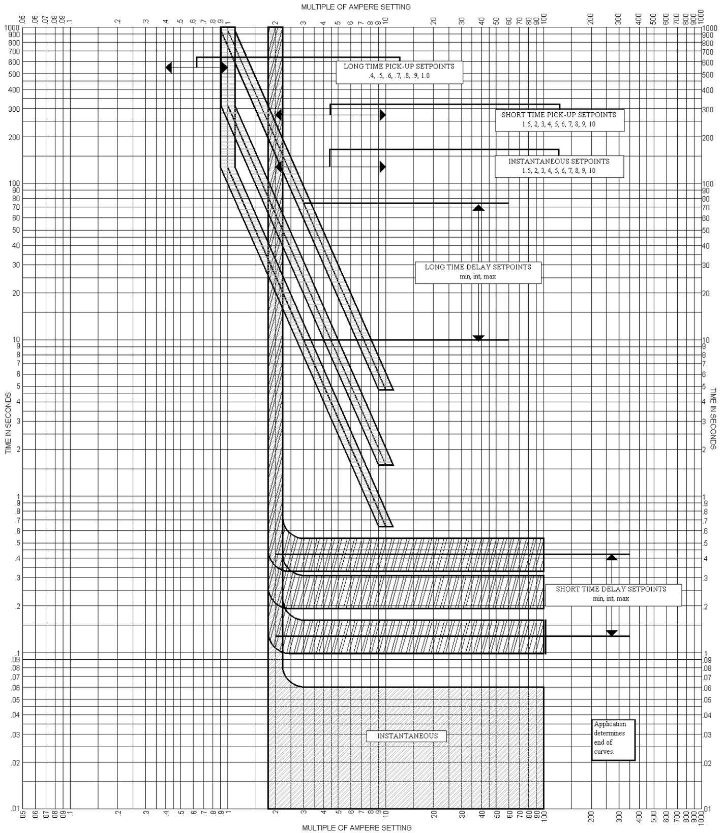
DC-2004 Programmable Logic Controller TIME-CURRENT CHARACTERISTIC CURVES
